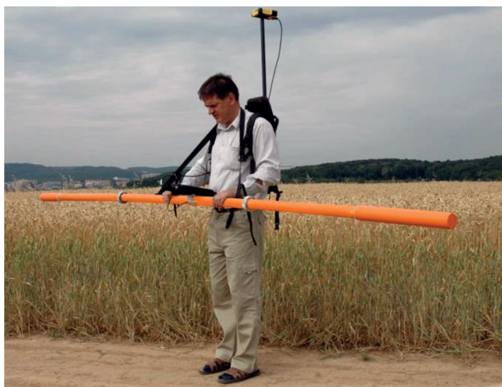
Fig. 2.1 Field measurements by CMD screening (source: www.gfstruments.cz )
