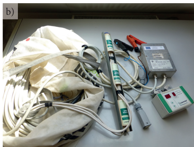
Fig. 1.11 (a) Automatic groundwater level and temperature measurement device plugged into a USB data reader; (b) 12 V DC centrifugal submersible sampling pumps Gigant GR 4 with regulation of flow rate
