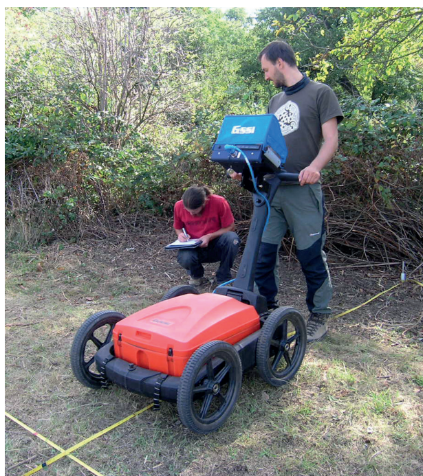
Fig. 2.3 Georadar measurement on designated geophysical profiles
