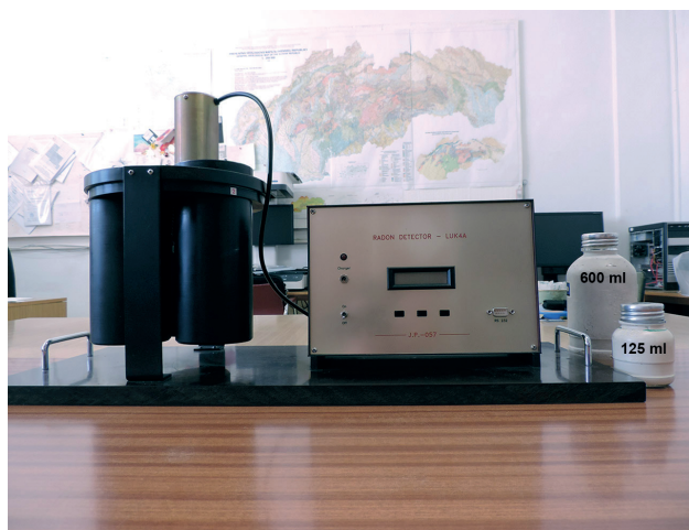
Fig. 2.7 Apparatus LUK-4 and Lucas Chamber volume 125 and 600 ml (source: www.geology.sk )
