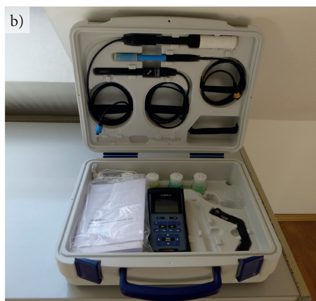
Fig. 1.9 Field measuring instruments: a) portable multimeter for measurement of pH, Eh, temperature, dissolved oxygen content and specific electrolytic conductivity, b) groundwater level meter enabling measurement of temperature and specific electrolytic conductivity of water
