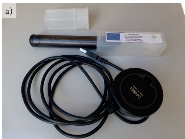
Fig. 1.11 (a) Automatic groundwater level and temperature measurement device plugged into a USB data reader; (b) 12 V DC centrifugal submersible sampling pumps Gigant GR 4 with regulation of flow rate
