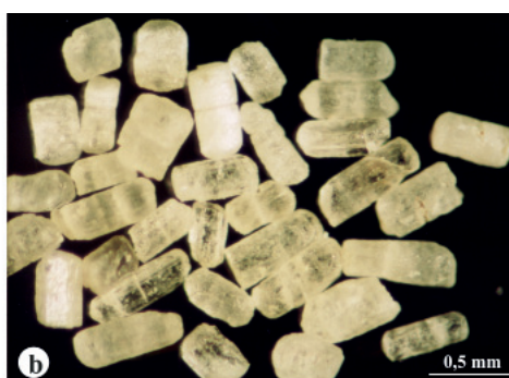
Fig. 4.8a, b, c Typical shapes and colour of apatite in the panned concentrate samples. On small crystals of apatite prismatic planes dominate with regular and identical habit (a) or irregular (c) one. The crystal termination can be characterised by dominant pinacoid shape (a) or the pyramid (c). Drawings: Rösler, J. H., 1983. Photo (b): P. Bačo.
