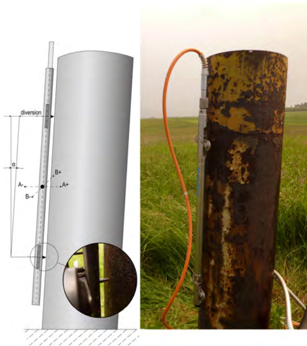
Fig. 7.8 Principle of measurements of change in angle of geodetic pillars by inclinometric probe
