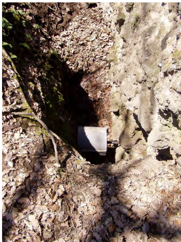
Fig. 7.25 Dilatometer TM-71 (KK-2) installed in the open crack between upper block and intact massif of the lava flow at the western margin of the stratovolcano Strechový vrch
