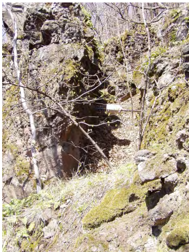
Fig. 7.24 Dilatometer TM-71 (KK-1) installed in the open crack between two (bottom and top) blocks at the western margin of the lava flow of the stratovolcano Strechový vrch
