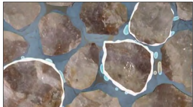
Fig. 2.5 Dense CO 2 migrating upwards (light blue bubbles), dissolving and reacting with the grains of the rocks. Leading to precipitation of carbonate minerals on the grain boundaries (white). (Source CO 2 GeoNet ).
