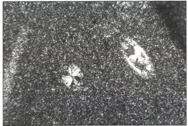
Fig. 6. Radiolaria shale of the Upper Triassic age. X polars, magn. 65x.
