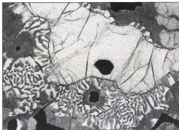
Fig. 11. Symplectitic eclogite composed of Gar, Cpx, Hbl, Ab, Rtl. X polars, magn. 75x.
