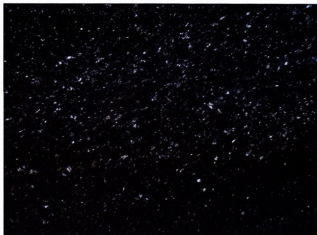
Fig. 2.D. - General view of the texture present in a vulcanite object. Crossed polars. Width of photo = 2,5 mm.
