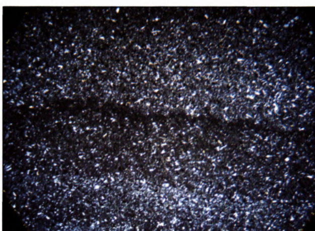
Fig. 9.D.- Micrograph of tin section of a gauge made in a volcanic tuff, lightly metamorphized. Alberite I Dolmen. Neolithic. Crossed polars. Width of photo = 6 mm.
