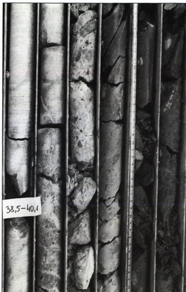
Fig. 4 Bobova Breccia at the base of the whitish sandstone of the Farkasnyak Sandstone Mb. of Szentlélek Fm., Middle Permian. Borehole Mályinka-13, (37,4-38,7 m), Csikorgó, NE Bükk Mts.
