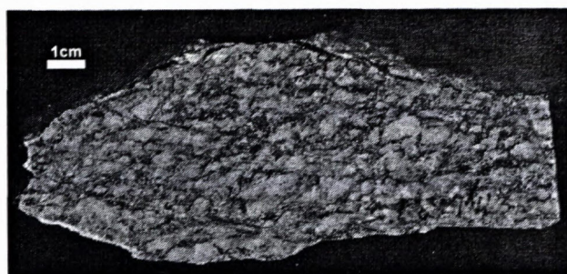
Fig. 5 Photograph of the protomylonite. Note the development of the "s" planes foliation. Malé Jastrabie locality.
