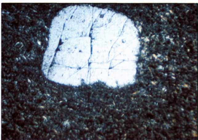
Fig. 17 Very fine-grained (0,1 mm) amphibole schist (after intermediate porphyritic volcanic rock). In the given rock sporadically plagioclases (up to 3 mm) occur. B-95a - shoe-last wedge. Crossed polars.
