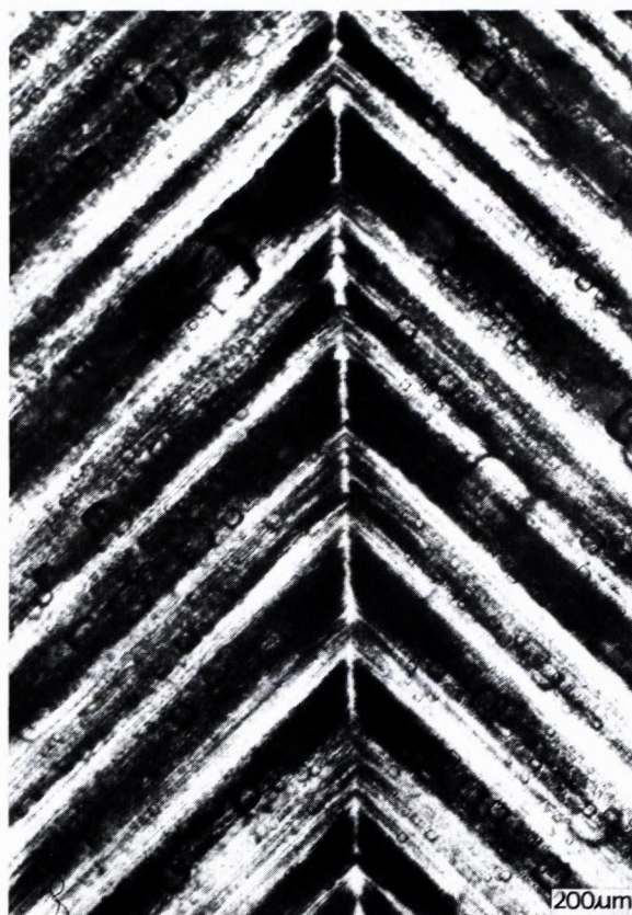
Fig. 4. Symmetric chevron crystal with definite rhythmic zonation.
