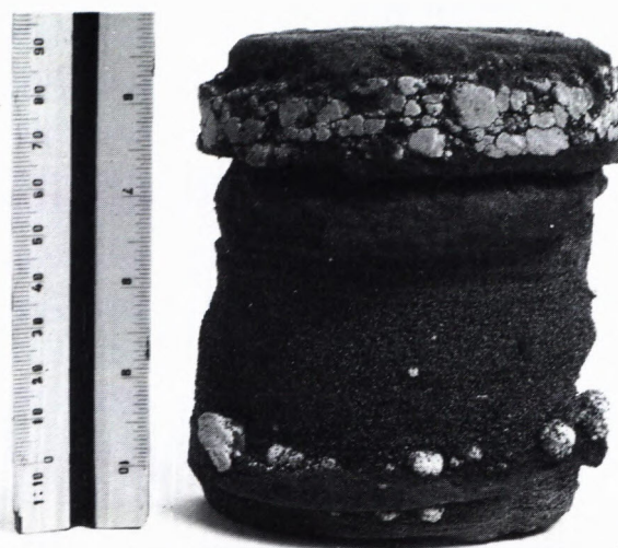
Fig. 8. A core of sandstone with graded bedding (white grains of anhydrite show the gradation from bigger to smaller ones towards the top of the layer, similar to the other components). Borehole no. 963.
