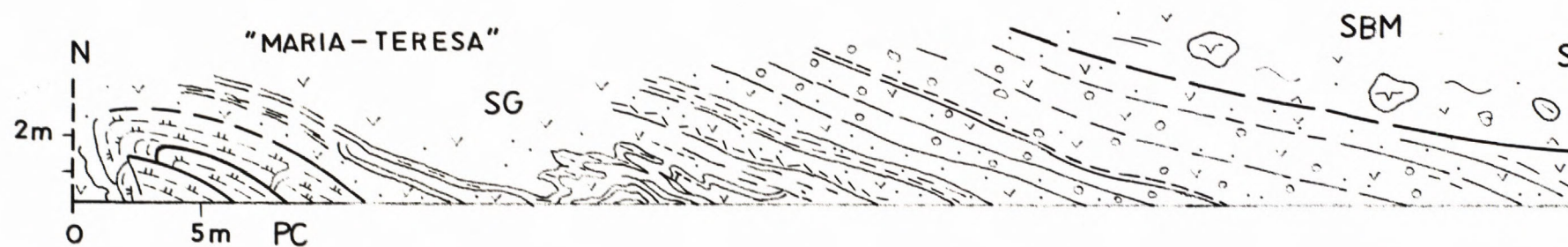
Fig. 9 (A) Cross-section through the folded Upper Spiza (SG) unit with salt conglomerates and contact with the overlying unit - Salt Breccia Member (SBM). Thrust-faulted Central Barren Intercalation rocks (PC) occur in the core of an anticline to the north. Maria Teresa Gallery.
