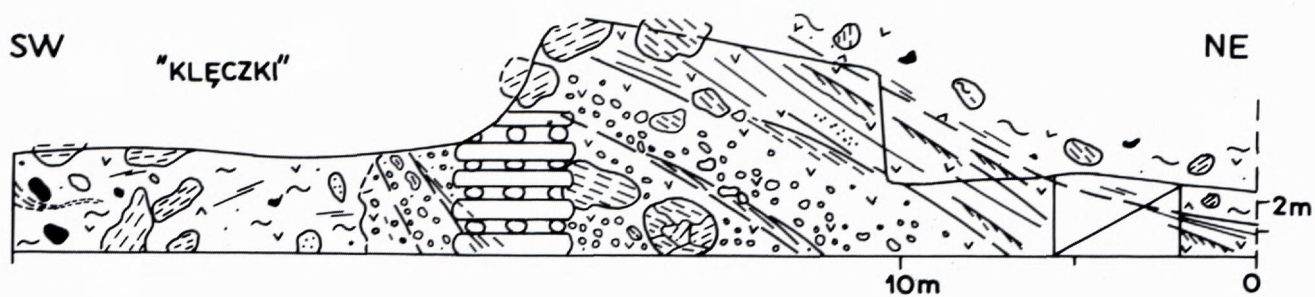
Fig. 20. Cross-section in the Kłęczki chamber showing the nature of the unit intercalated between two mega-debrites in the Salt Breccia Member. The intercalation here comprises graded salt conglomerates terminated by cross-bedded saltstones.
