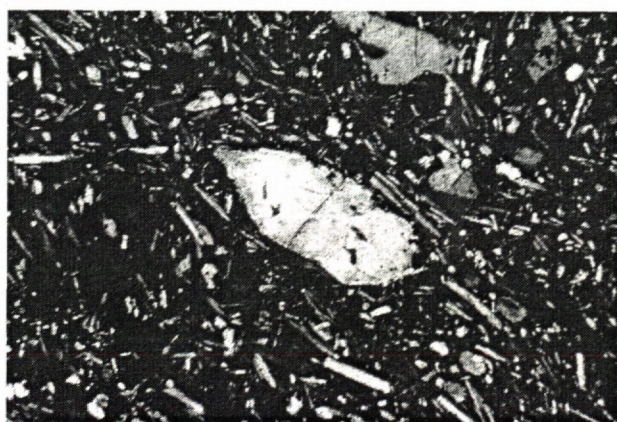
Fig. 2 Poorly expressed fluidal pattern of an alkali basalt. In the middle of the micrograph the olivine phenocryst: plagioclases have a lathy morphology. Thin section: S - 27, X polar. magn. 90x (by Hovorka et al., 2000).
