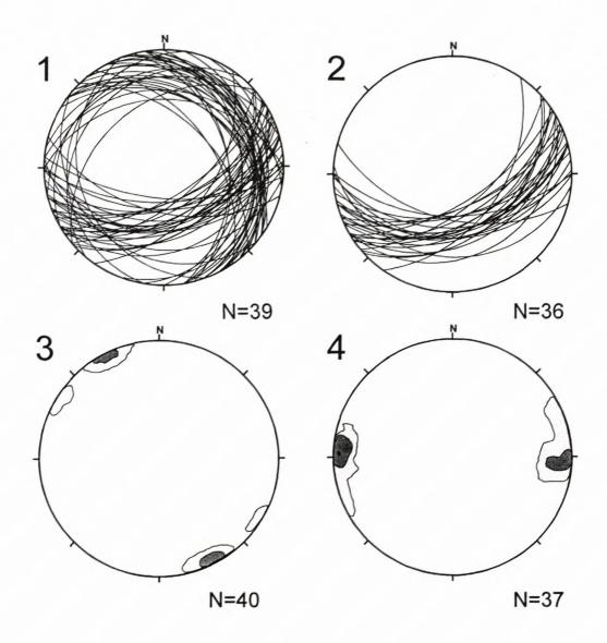
Pl. V. Great Circle (Equal area, lower hemisphere projection) and Contour orientation diagrams of mesostructures of the VZP Complex. 1 - Magmatic  $S_0$  and mylonitic/metamorphic foliation planes  $S_1$ . 2 - Alpine extensional cleavage planes  $S_2$ . 3 - Lineations of magmatic flow  $L_0$ , and mylonitic/metamorphic lineations  $L_1$ . 4 - intersection lineations  $L_2$ .
