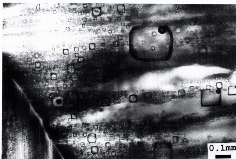
Fig. 4. Fragment of chevron structure in halite in part with rhythmic zonation. Inclusions are liquid with gas bubbles. Transcarpathians, Mukacheve depression, borehole 6-T, depth 1074 m.
