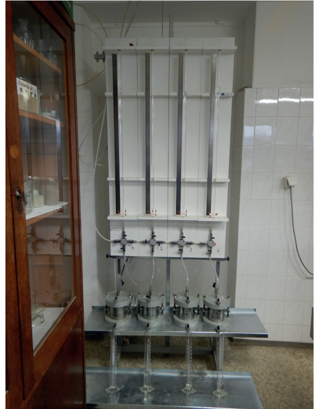
Fig. 4.3 Permeameter for constant and falling head test
