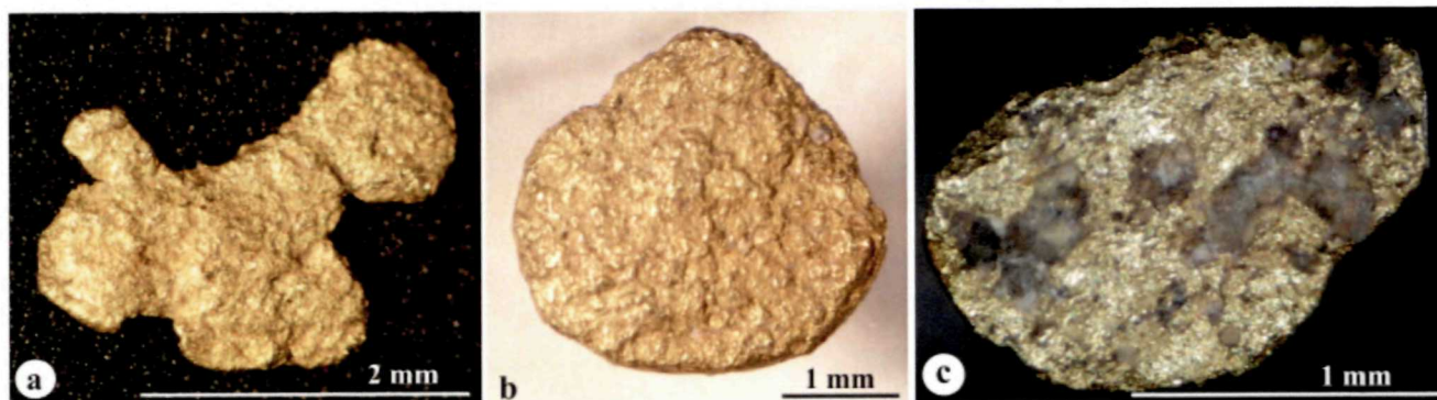
Fig. 4.91a, b, c Colour and lustre of gold in the panned concentrate samples. Colour and shades are dependent on impurities, mainly Ag. At its high content it has dark-yellow colour, at Cu-content it turns to reddish-yellow hue. Part of gold flakes can be coated by Mn- and Fe- oxides. Site: a – c Ruská Bystrá. Photo: P. Bačo.
