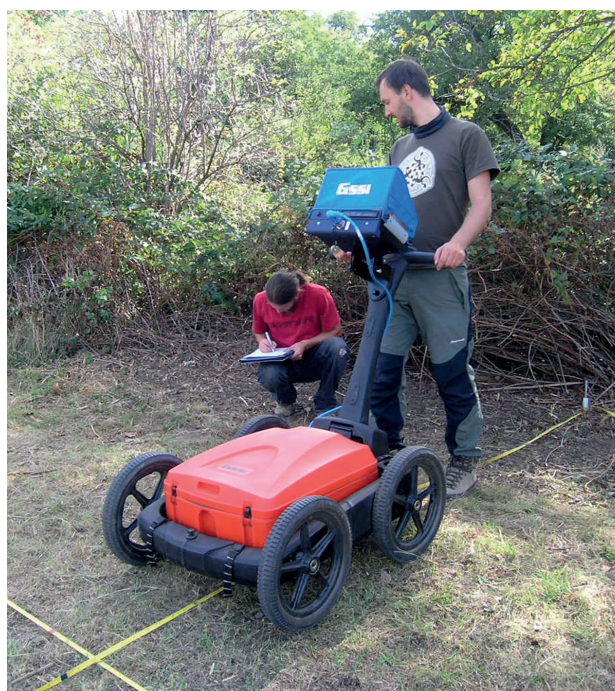
Fig. 2.3 Georadar measurement on designated geophysical profiles
