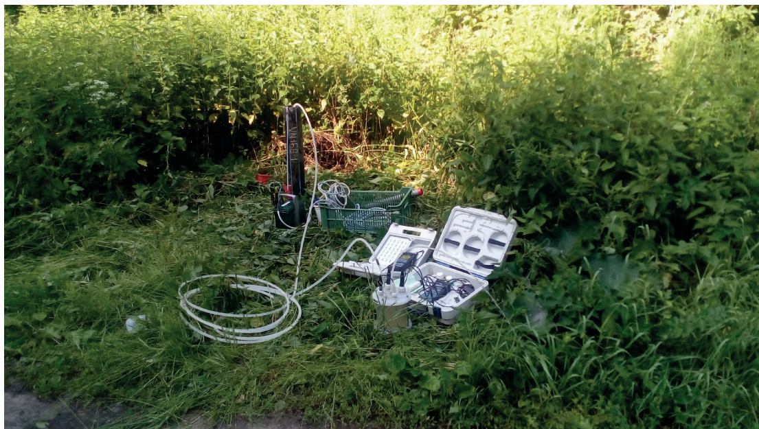
Fig. 1.10 Sampling and measurement of indicators using multimeter and flow cell
