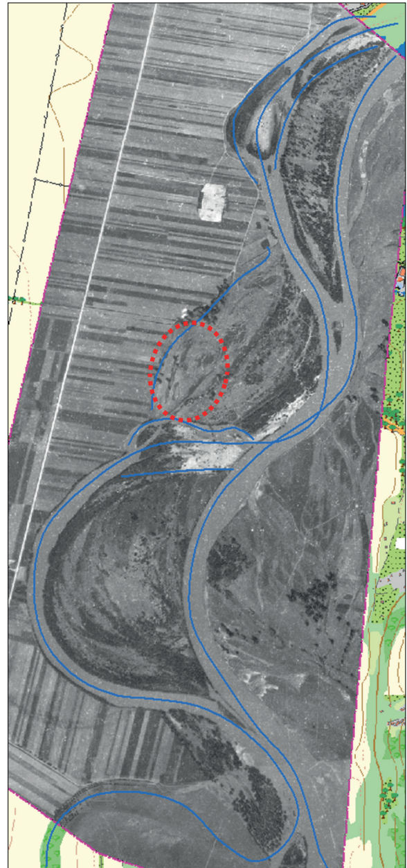
Fig. 3.3a Location of the future EB on a historical aerial photograph from 1950 (an old oxbow flows right through the site of the river Váh – marked with blue colour)
