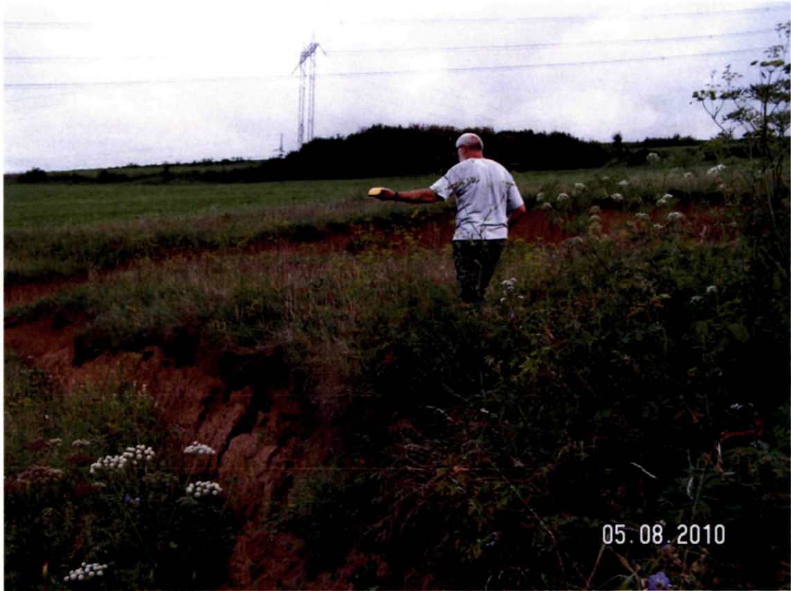
Fig. 3.2 GPS recording of landslide main scarp in Spišské Vlachy village, during the field survey and mapping of new activated landslide after rapid rainfall event in June of 2010.
