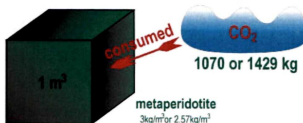
Fig. 7.11. Scheme of the volume of sequestered CO 2 in 1 m 3 of metaperidotite.
