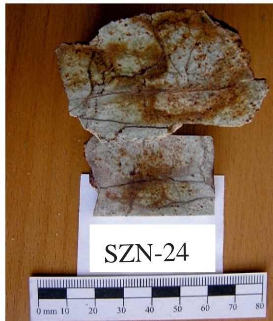
Fig. 8. Sample of tremolite-plagioclase rock with deficiency of dark minerals. In the field this rock resembles the fine-grained quartzitic rock (sample SZN-24).
