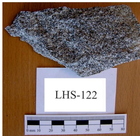
Fig. 42. Fine-grained omnidirectional, grey biotite-rich microgranodiorite-microtonalite, as one part of the biotite granodiorite-tonalite body (sample LHS-122 – Krstenica valley).
