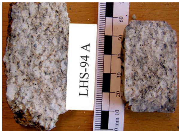
Fig. 32. The medium-coarse-grained, more leucocratic types of granodiorite rocks with irregular spatially and size-distributed biotite.
