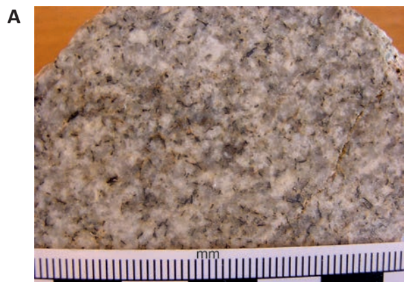
Fig. 35. Different types of planar oriented leucogranites: A – Planar oriented two-mica granite in the subsolid stage, with a pegmatite vein without deformation (sample LHS-626). B – Planar oriented two-mica granite with developed subsolid quartz bands (sample LHS-623).
