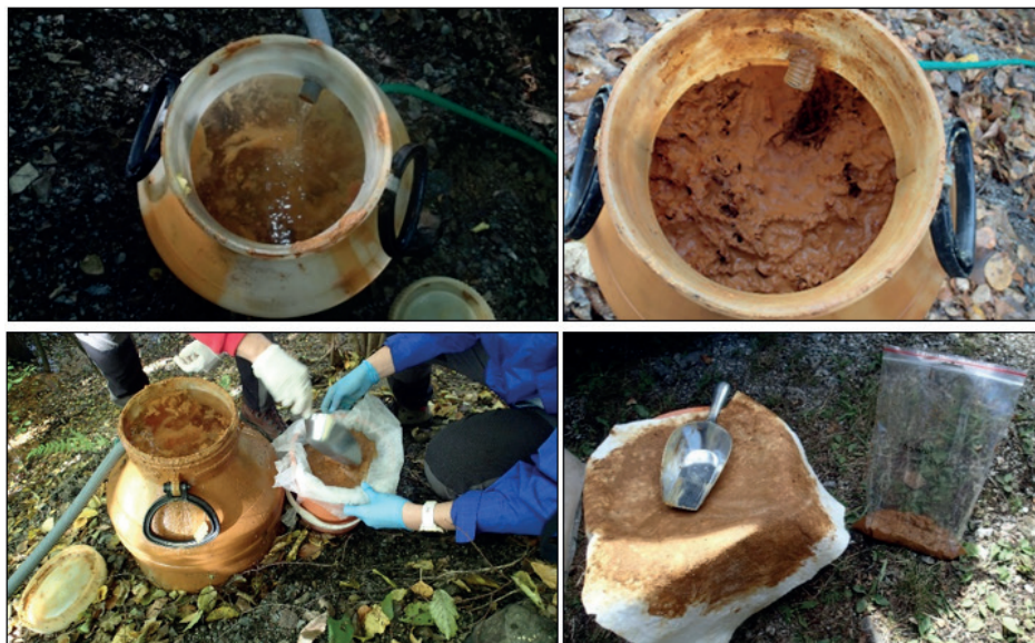
Fig. 3. Formation of ochre precipitates in a 50 L sedimentation container, ochre sampling.
