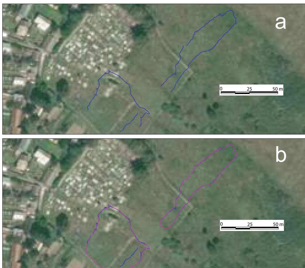
Fig. 1. Accuracy of GPS measurements – class 1. a – rough line of GPS measurement; b – the same line smoothed.
