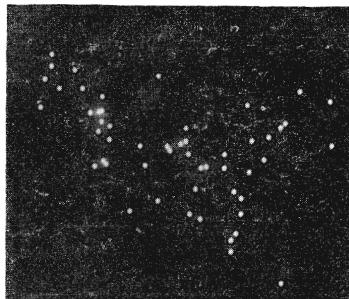
Obr. 15. Distribúcia Ag( L_\alpha ) v uzavrenine Fig. 15. Distribution Ag( L_\alpha ) in the inclusion. Electron microprobe analyzer
