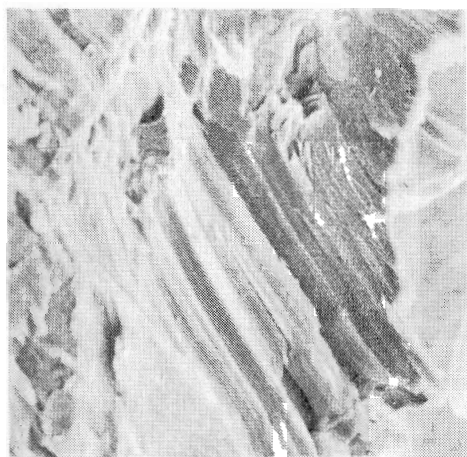
Fig. 18. Prevalence of tabular-columnar lizardite over chrysotile (sample 4a, Jaklovce). Scanning microscope, magnif. 500 \times
