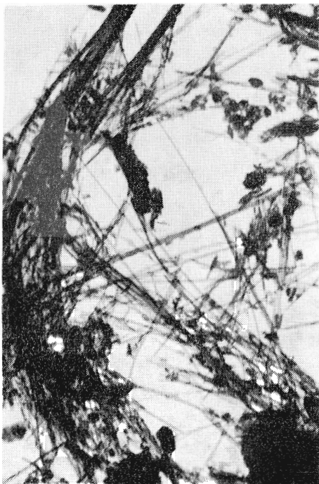
Fig. 16. Vein chrysotile fiber accumulations (sample 17, Jaklovce). Magnif. 7000 \times , TEM
