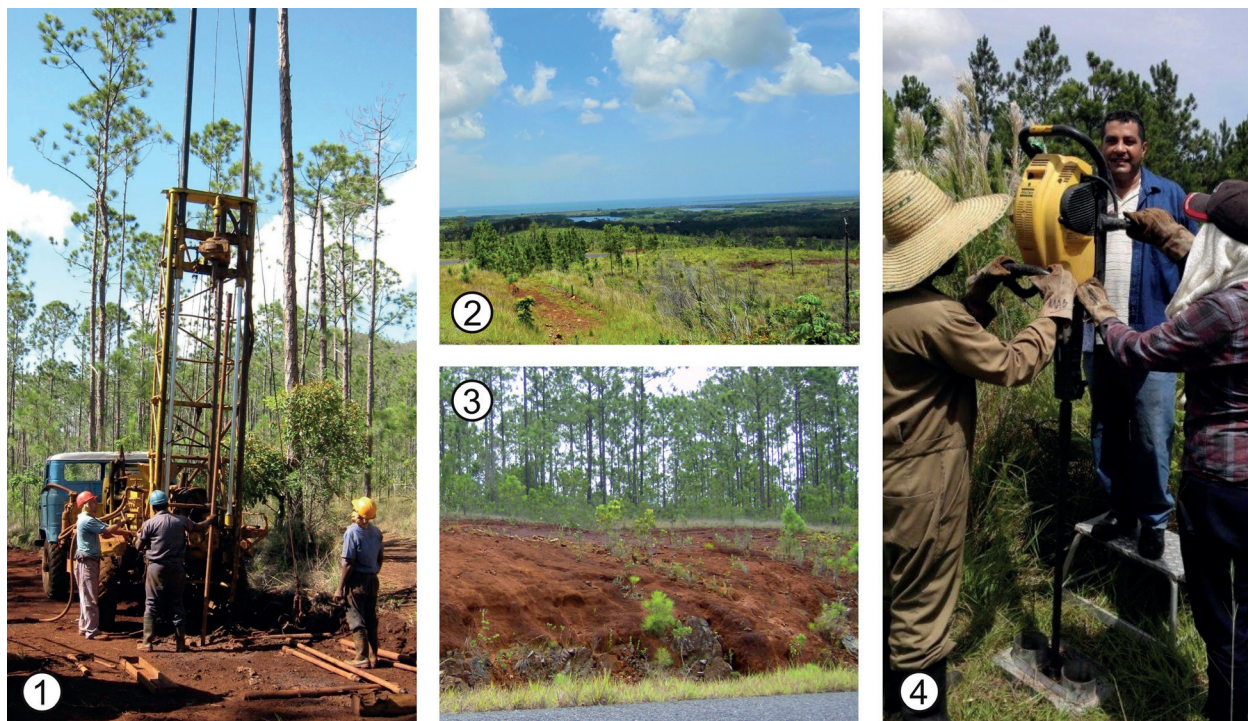
Fig. 1. Exploration in the Cajálbana laterite deposit. 1 – Drilling facility UGB-50 with drilling capacity up to 100 m with spiral drilling and 65 mm of diameter, 2–3 – Cajálbana area is typical with red lateritic soil and contains traces after exploration works, 4 – complementary drilling for limonitic ore applying the Atlas Copco portable drill.
