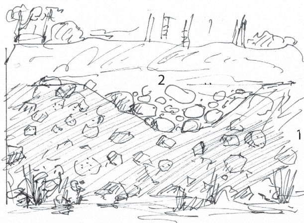
Fig. 37. On the southern slope of the Pokoradz Plateau of the Stráň locality at level 510 m a.s.l., the chaotic breccia of pyroclastic flow is exposed (1 in scheme). Breccia consists dominantly of vesiculated subspheric fragments large 5–20 cm and rarely by angular blocks of dimensions up to 30 cm. On the surface of chaotic breccia, the erosive channel is filled by the coarse conglomerate material (2 in scheme). The erosive channel on the surface of chaotic breccia of the layer-4 documents continuing processes of erosion and destruction of chaotic breccia in the littoral zone occurring immediately after deposition of pyroclastic flow.
