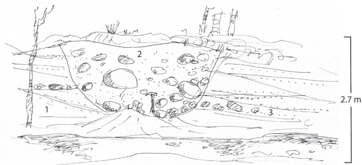
Fig. 14. Bed of epiclastic volcanic sandstone exposed in the forest cut (at the eastern edge of the Pokoradz Plateau below e.p. 491 west of Dražice village. Medium to coarse epiclastic volcanic sandstone is distinct with cross bedding structures (1) and frequent lenses of fine andesite conglomerate (3). Erosive channel (2) cut in epiclastic volcanic sandstone is filled with the coarse to blocky epiclastic volcanic conglomerate.
