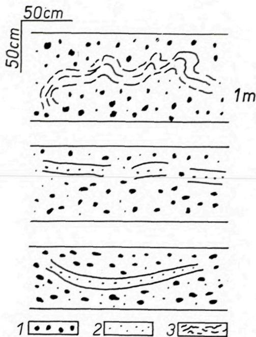
Fig. 3. Detail structure of the slump body, locality Údavské, 1. Conglomerate, 2. Sandstone, 3. Claystone.
