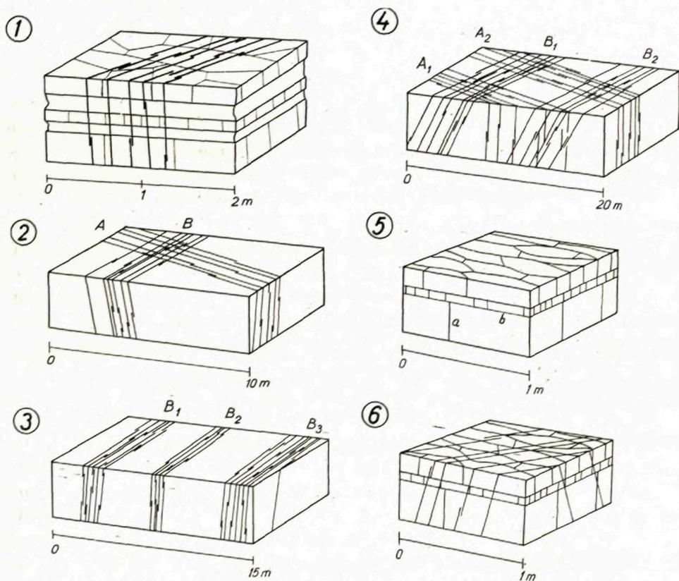
Fig. 1. Block diagrams showing schematically joint zones and bedding joints
