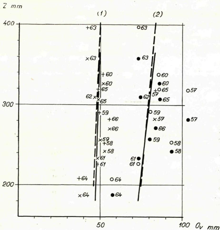
Fig. 3. Dependence of the total discharge of springs from carbonate complexes of the Choč (1) and Krížnan (2) units in Small Carpathians from November till April ( $O_v$ ) on the sum of rainfall ( $Z$ ) for the same period (1957–1966)
