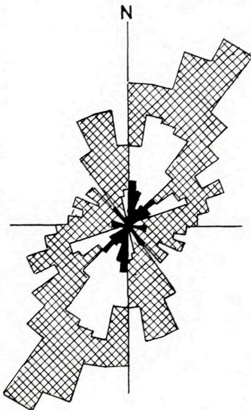
Fig. 1. Rose diagram of strikes of the faults of the Štiavnica Horst. checkered — 165 dykes of hornblende-biotite dacite; plain — 57 ore veins; solid — 44 faults (mostly without mineralization)
