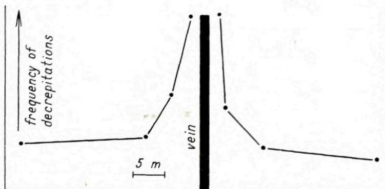
Fig. 8. Frequency distribution (ordinate) of decrepitations in the vicinity of a hydrothermal vein in granite.
