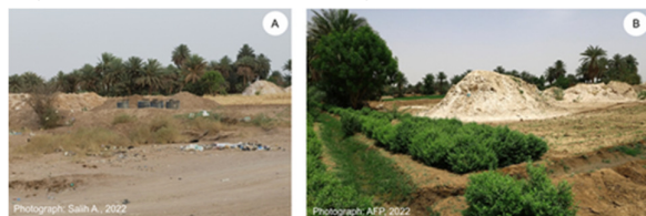
Figure 2 Mining tailings and thiourea-based extraction unites inside the farms alongside the Nile River.
