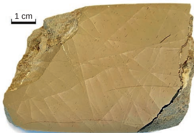
Fig. 3. Light brownish-grey marlstone to limestone (so-called “treskúň” or “ruin marble”) from the 25–25.5 m interval.
