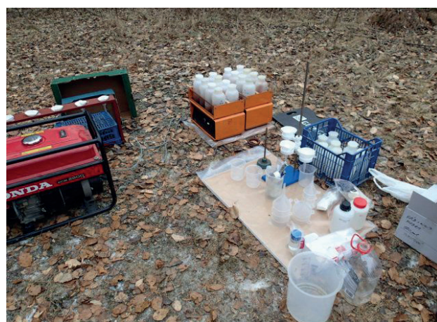
Fig. 14. In-situ batch adsorption experiment.
