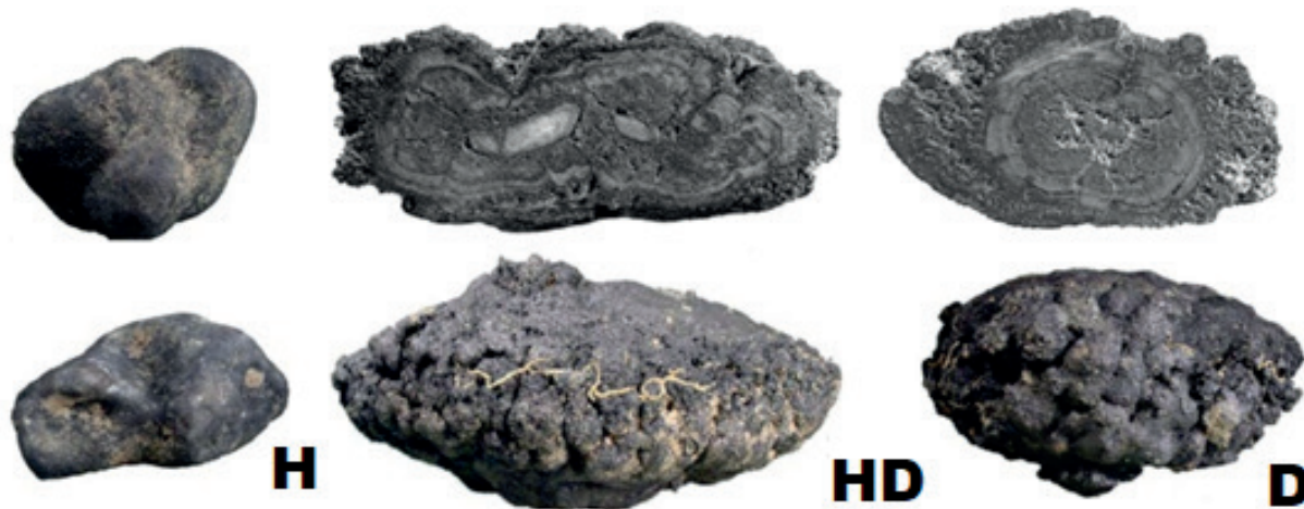
Fig. 9. Main genetic types of nodules: H – hydrogenetic (smooth surface), HD – combined (smooth surface on top, rough from below) and D – diagenetic (rough surface) (Kotliński, 2011).
