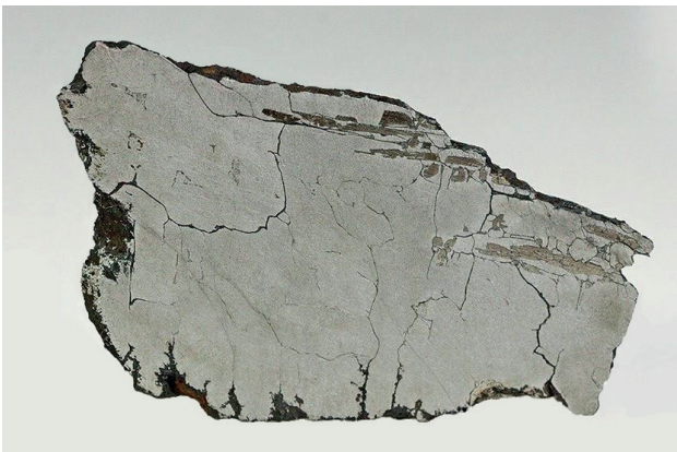
Fig. 2.2 Up to 2 cm long longitudinal lobular aggregates of the cohenite in the Magura meteorite. Photo: D. Ozdín
