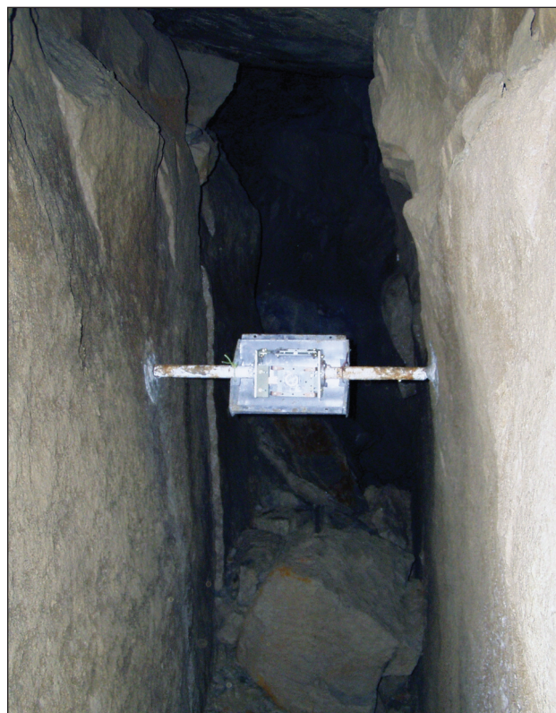
Fig. 6. Installation of the TM-71 extensometer inside one of the main passages of the Cave under the Spišská hill (behind the place called Crossing). The NE–SW oriented passage (footwall) has inclination of 12°. Photo by Petro (2007).
