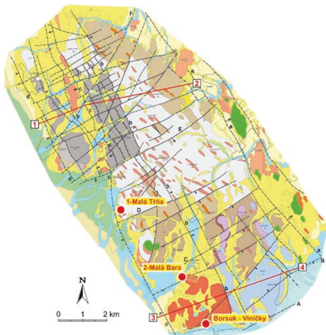
Fig. 2. Tectonic scheme of the Zemplínske vrchy Mts. (Kobulský and Gazdačko in Kobulský et al., 2011) with position of localities 1 and 2, as well as the position of volcanic body Borsuk. Tectonic scheme indicates the principal overthrusts and faults. Two dominating trends of faults were revealed: Faults of NW–SE direction: a – Somotor fault; b – Viničky fault; c – Trňa fault; d – Čerhov fault. Faults of NE–SW direction: A – Poľana fault; B – Kapušany fault; C – Zemplín fault; D – Cejkov fault; E – Kašov fault; F – transversal Hrčel fault. The detail information about the lithology is available comparing two cross-sections in Fig. 3.
