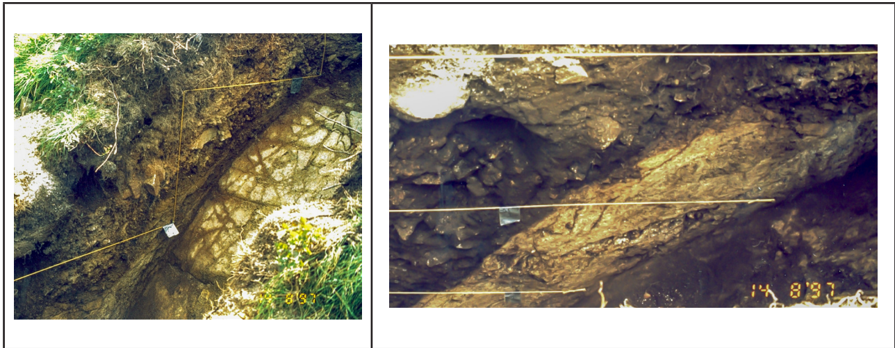
Fig. 9. Photographs of the main fault zone in Trench 2. Left – fractured granodiorite of the fault footwall at lower right. Shear zone is visible below lower string line. Right – closeup of shear zone. String lines are 50 cm apart.
