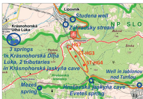
blue rings - detection sites in 11 monitored locations around the route, red rings - tracking application in 3 tunnel boreholes
