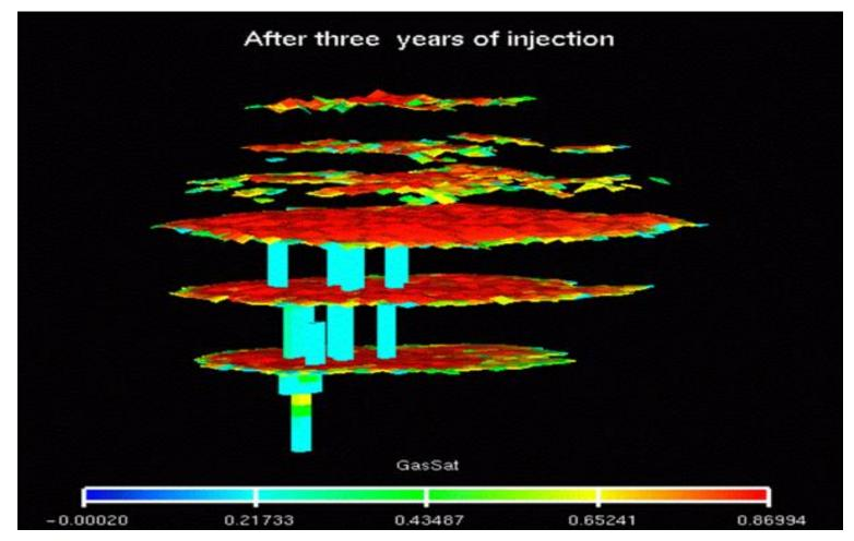
Simulated picture of the distribution of  $CO_2$  after three years. Radius of largest bubble 800 m and the total plume 200 m high.
