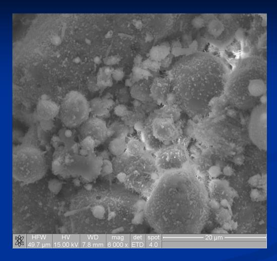
Noticeable ash grains covered with microcrystalline silicates hydration, distinguishable calcite
